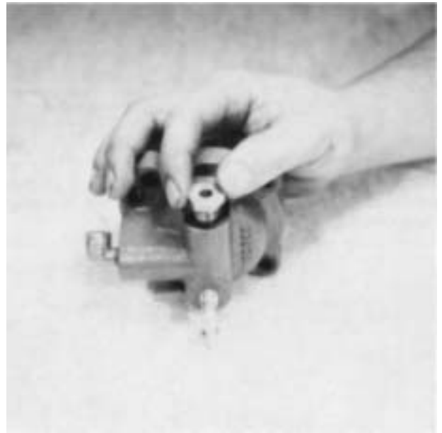
9. Install the exhaust screw in the cover to retain the insert valve.
