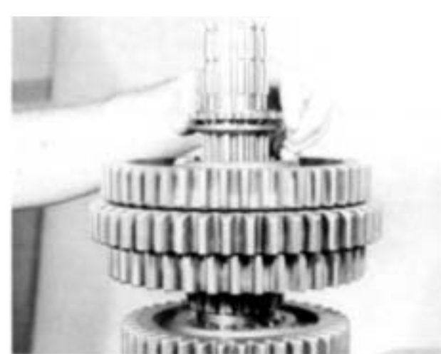
18. Install the spacer, flat surface down.
