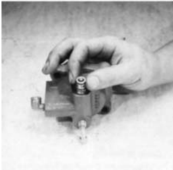
8. Install the insert valve in the cover as shown.
