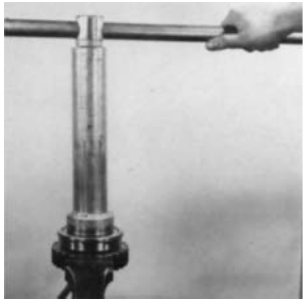
3. Relieve the bearing nut where it is peened into the shaft and turn the bearing nut from the shaft; left hand thread.
