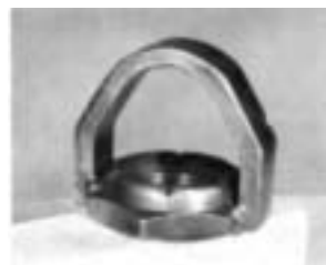
OUTPUT SHAFT HANGER BRACKET Make from yoke stop nut and flat steel stock.
