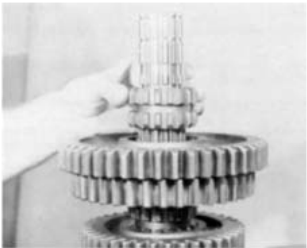
15. Install the sliding clutch, aligning the keyway over the key.
