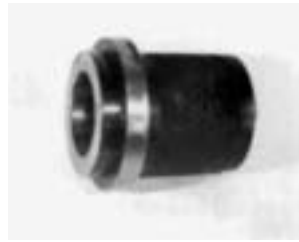
OIL SEAL DRIVER Print Number T-18088-23 Used to install the oil seal in the rear bearing housing.
