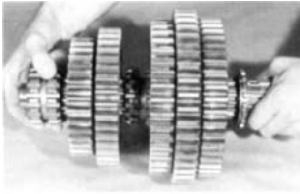
20. Remove the assembly from the vise and install the sliding clutch.
